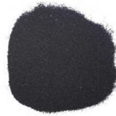
Fig. 2 Crumb rubber used in this research
