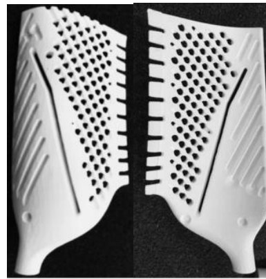
Fig. 7 Ceramic core for the blade
