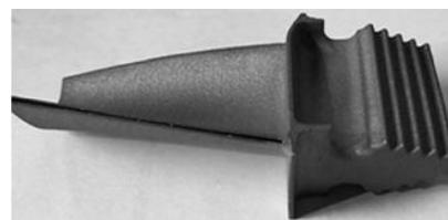
Fig. 8 The blade manufactured by DMLS technology
