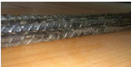
Fig. 4 Cleaned rebars after corrosion
