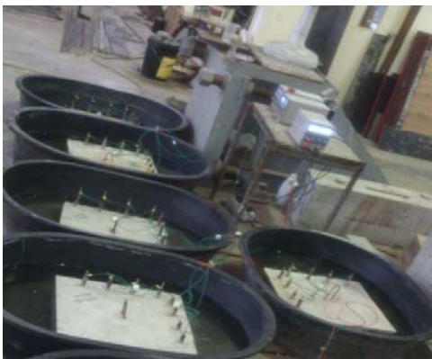
Fig. 1 Accelerated corrosion apparatus for slab elements
