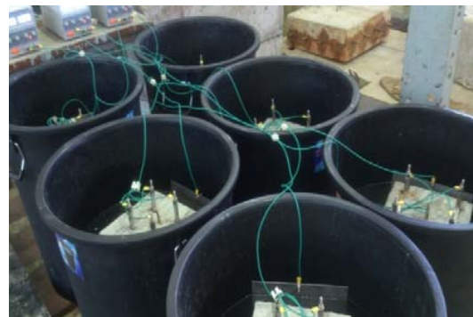
Fig. 2 Accelerated corrosion apparatus for column elements
