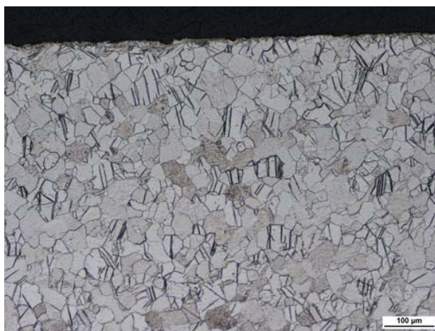
Fig. 3 The initial structure of Ti Grade 2 with the mean grain size of 62 μm
