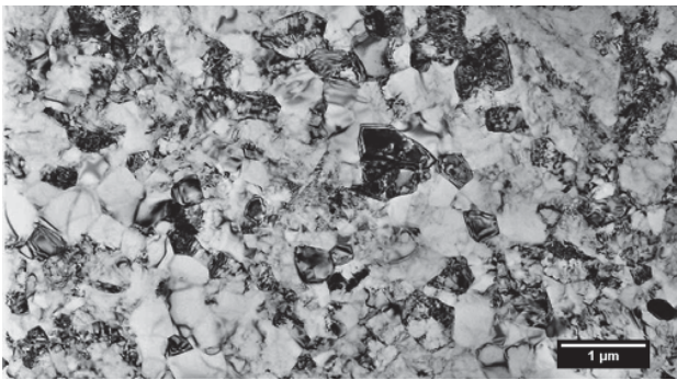
Fig. 5 The structure of Ti Grade 2 upon three passes through CONFORM SPD; the mean grain size is 390 ±150 nm
