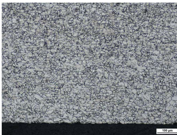
Fig. 4 The initial structure of Ti Grade 4 with the mean grain size of 32 μm
