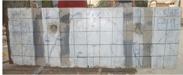
Fig. 10 Crack pattern of beams with opening above NA
