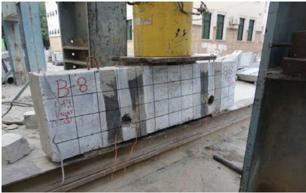
Fig. 5 Loading arrangement for beam testing
