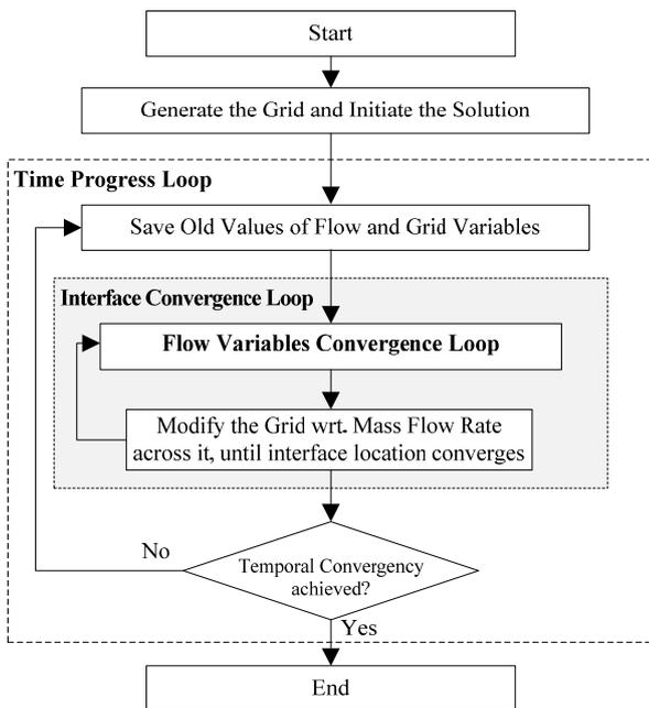
Fig. 6 Numerical solution algorithm for interface tracking
