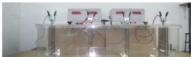
Fig. 4 Experimental setup used for the application of the electrochemical method
