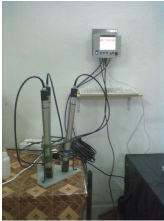
Fig. 5 The multi-parameter meter used for the monitoring of the pH, redox potential, and temperature
