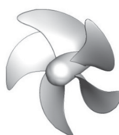
Fig. 1 Geometry of the Seiun Maru HSP propeller
