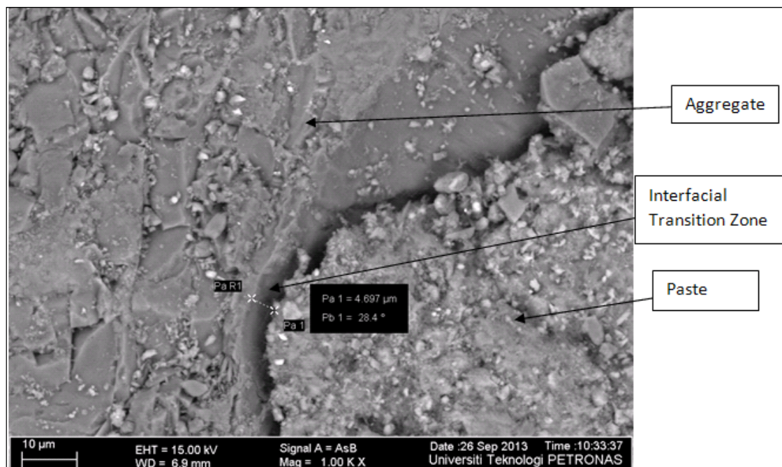
Fig. 5 Microstructure of concrete C-0 through FESEM
