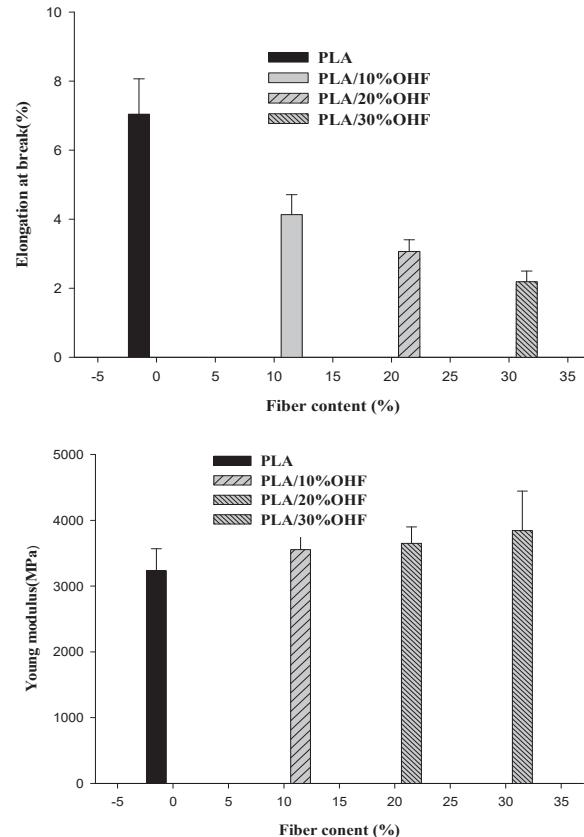
Fig. 2 Young modulus and elongation at break of composites at different fiber loading
