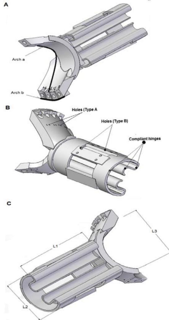
Fig. 3 The main features of the Palm-Socket module
