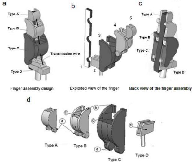
Fig. 2 Finger assembly and their stiff parts design
