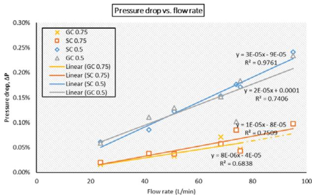
Fig. 14  $\Delta P$  vs. flow rate graph
