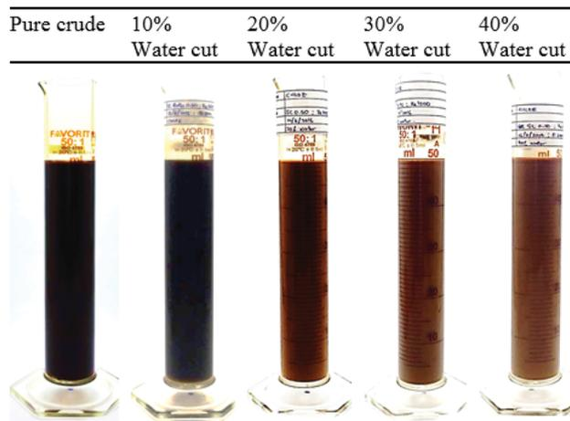
Fig. 9 Initial condition of the crude oil
