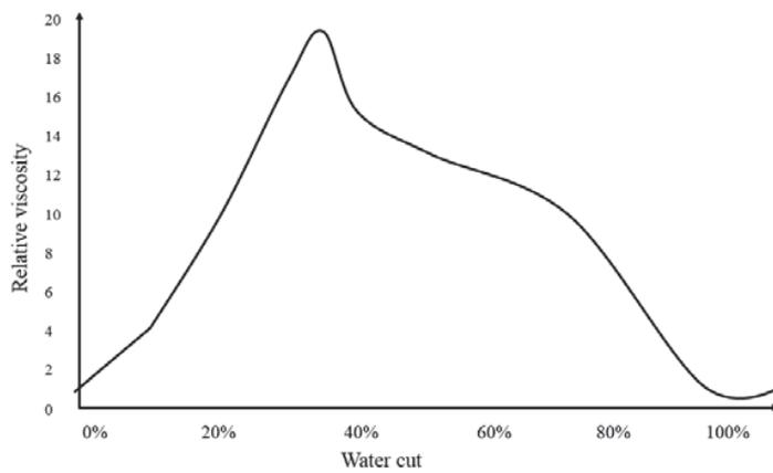
Fig. 3 Measured relative viscosity of different water cut [7]
