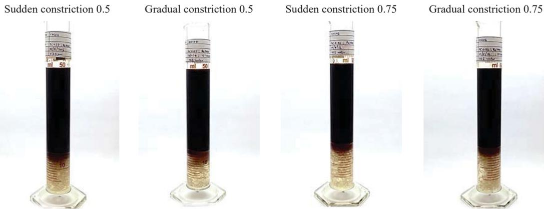
Fig. 10 Condition of 40 % crude oil after separation
