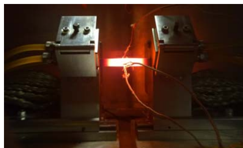
Fig. 2 Sample with thermocouples during heating
