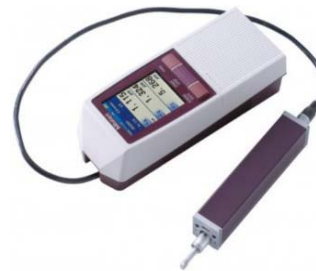
Fig. 3 Roughness meter used to measure surface roughness
