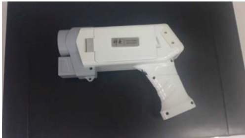
Fig. 8 Diagram of the portable ultrasonic leak detector
