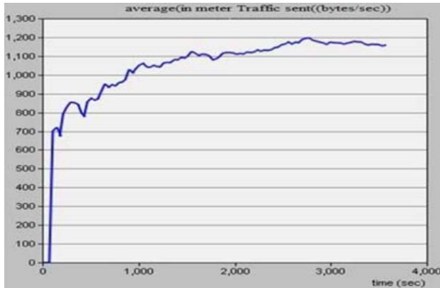
Fig. 4 Average WiMAX Throughput of Single Smart Meter
