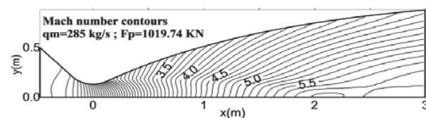
Fig. 2 Mach number contours in the nozzle
