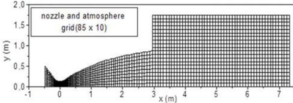
Fig. 3 Computational grid for  $P_a = 1$  bar
