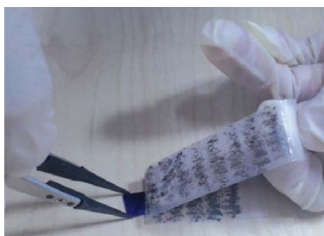
Fig. 4 Scotch tape method of graphene block [20]
