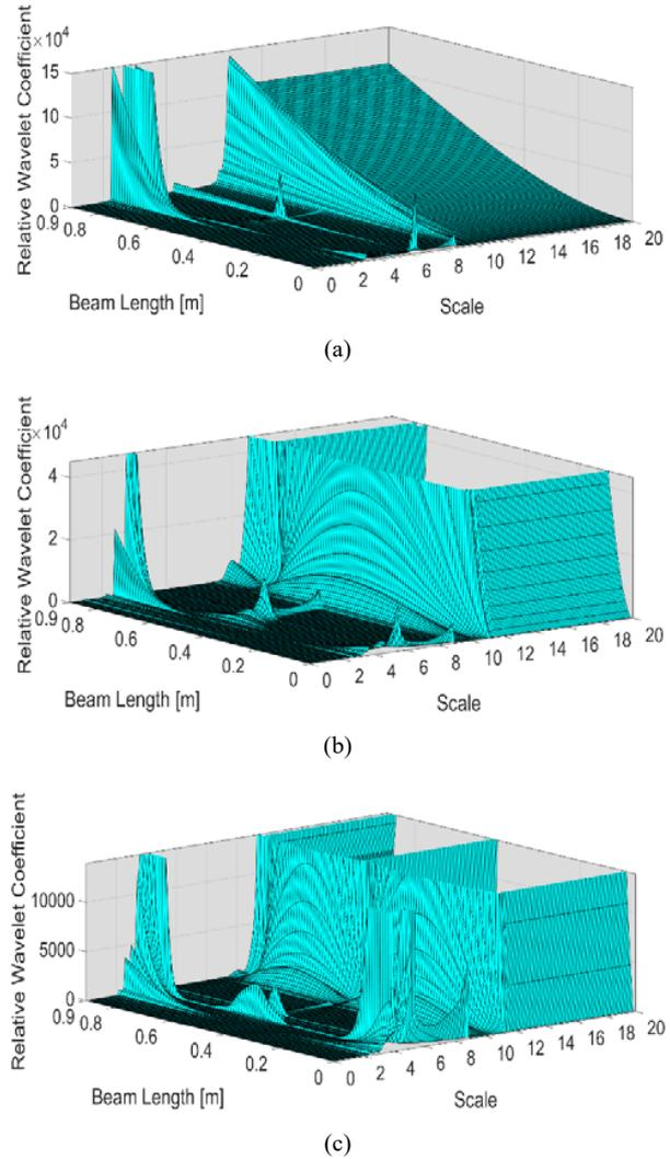
Fig. 2 Relative wavelet coefficient of the first three mode shapes with different scale factors at different positions of a beam with a crack at the middle (Crack depth = 0.125\*Beam height). (a) first mode shape. (b) Second mode shape. (c) Third mode shape
