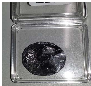
Fig. 5 Image of metallurgical silicon wafer obtained SX1744
