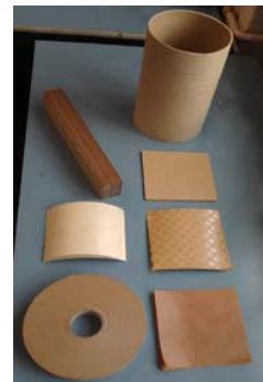
Fig. 1 Different types of transformers insulation material
