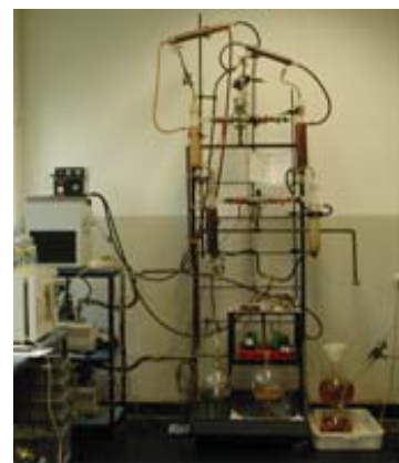
Fig. 2 (a) Schematic diagram and (b) picture of the drying system for insulating fluids
