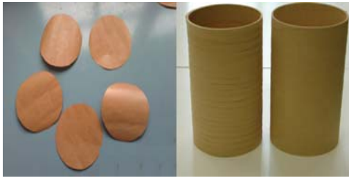
Fig. 4 Example of insulation paper samples
