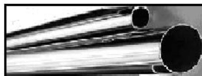
Fig. 2 Tube draft (before annealing) and finished tube (after annealing)
