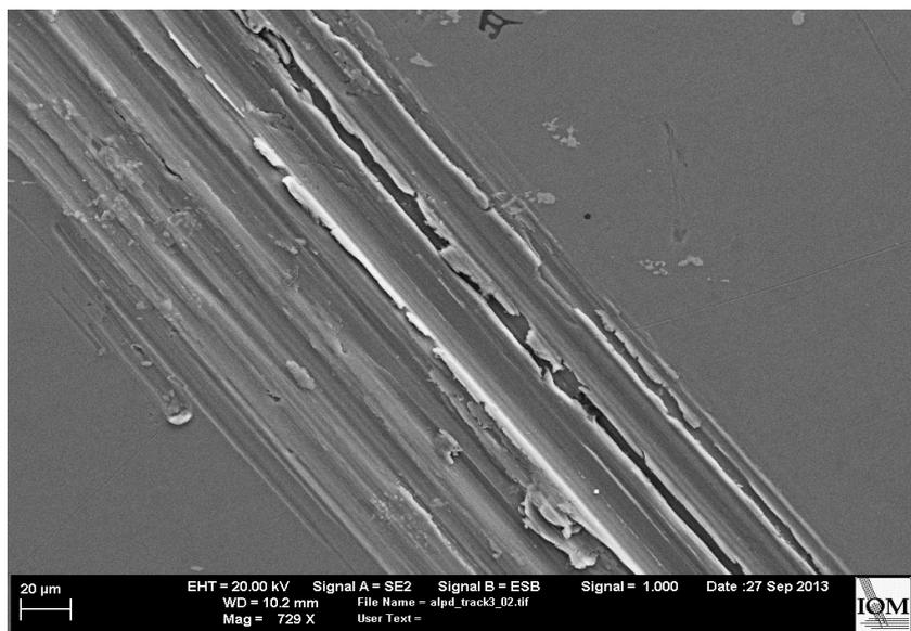
Fig. 3 (a) Friction coefficients, (b) tracks of untreated 7075 AA samples after 100 cycles, and (c) tracks of untreated 7075 AA samples after 50 cycles
