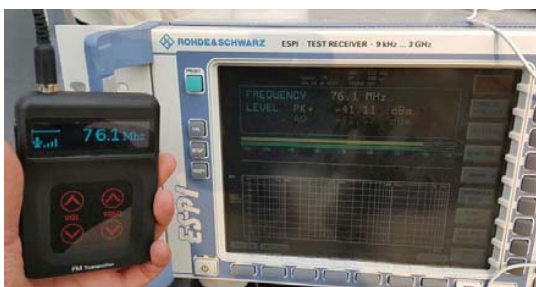
Fig. 9 Implementation result of embedded FM transmission control SW
