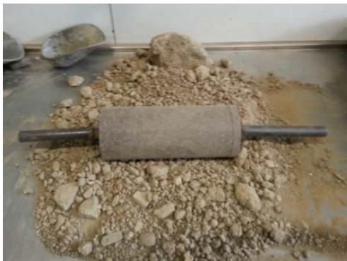
Fig. 4 Grinding the sediments after oven drying
