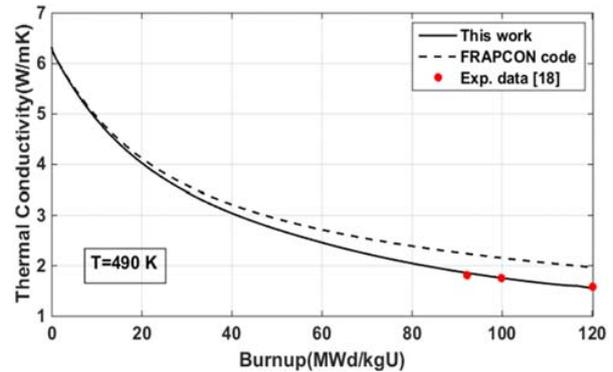
Fig. 3 Calculated  $UO_2$  fuel thermal conductivity based on FRAPCON code model vs. burn-up at 490K with porosity evolution included in comparison with the case with constant porosity and experimental data [18]
