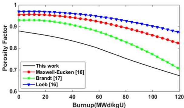
Fig. 2 Comparing the proposed porosity factor in (6) with others at 800K
