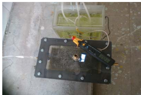
Fig. 3 The microbial fuel cell built for this research
