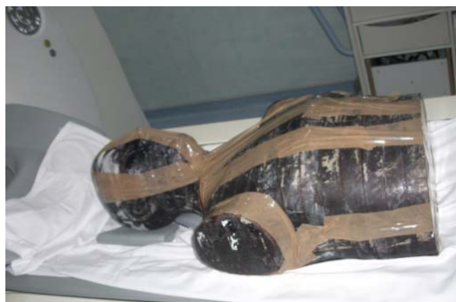
Fig. 1 Photograph of the RANDO anthropomorphic phantom in the Siemens Definition Edge 128-slice CT scanner
