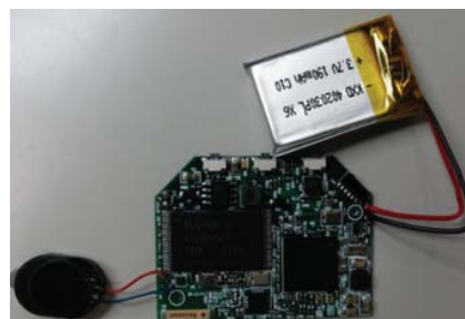
Fig. 4 The PCB module of the wearable guide device
