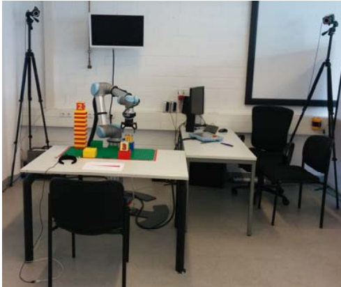
Fig. 2 Experimental setup, UR5 robot with gripper, screen, hairband with IMU, and motion capture cameras
