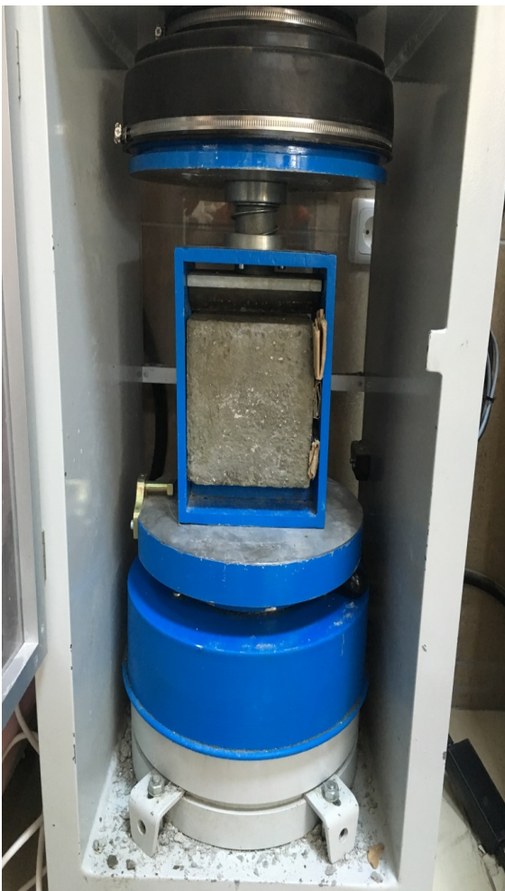
Fig. 5 Compressive strength test equipment
