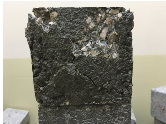
Fig. 3 Specimen after compressive strength test
