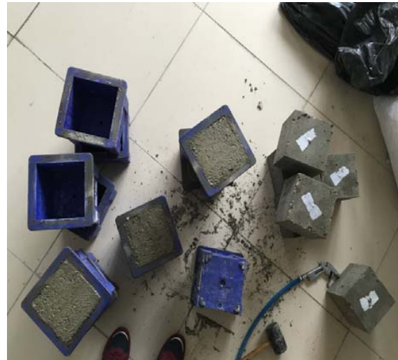
Fig. 6 Cube specimens after abstracting
