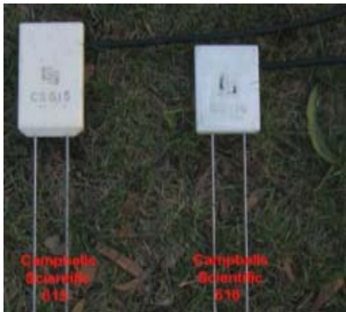
Fig. 4 CS-616 soil moisture probe [25]
