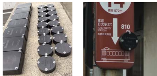
Fig. 2 Beacons (a) two kinds of beacons (b) a beacon on the pole
