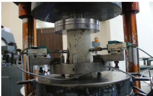
Fig. 3 Uniaxial compression test setup
