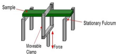
Fig. 2 Three-point bending configuration [33]
