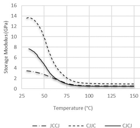
Fig. 3 Storage modulus curves of samples
