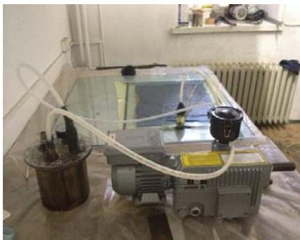
Fig. 1 Vacuum bagging system set-up
