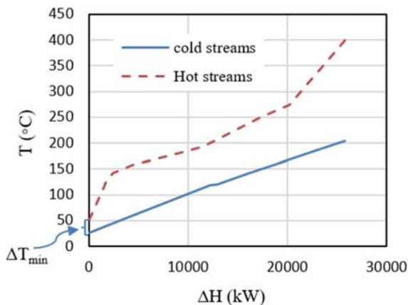
Fig. 4 Composite curve of the existing HEN
