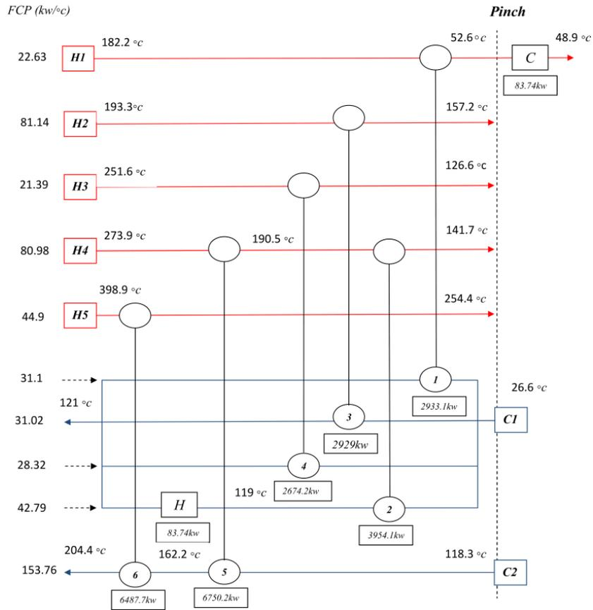
Fig. 7 Diagram of HEN for  $AT_{min}=26\text{ }^{\circ}\text{C}$
