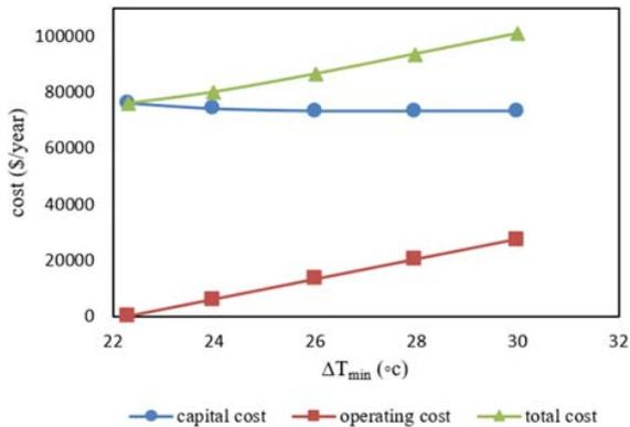
Fig. 10 Costs diagram based on  $\Delta T_{min}$
