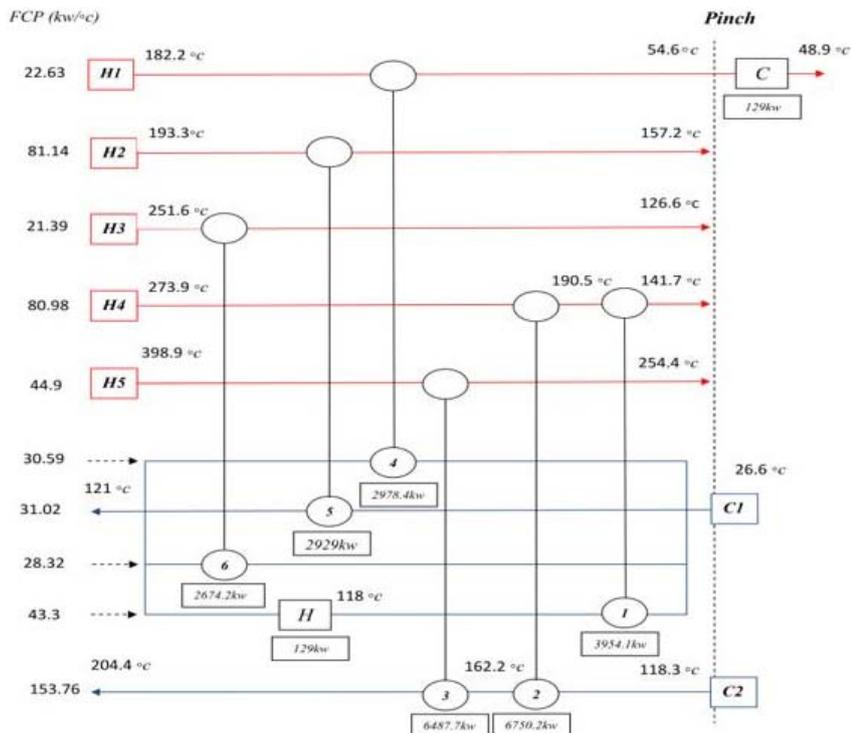
Fig. 8 Diagram of HEN for  $AT_{min}=28\text{ }^{\circ}\text{C}$
