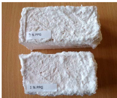
Fig. 7 Geopolymer mortar specimens containing 1 and 2% of PPG
