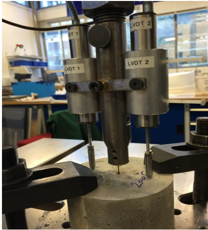
Fig. 2 Single fibre pull-out test setup
