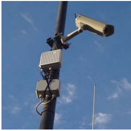
Fig. 7 An installed smart camera and the ETSI MSM Gateway installed on an existing pole during Montecatini trial
