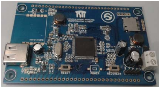
Fig. 8 The smart camera main electronic board
