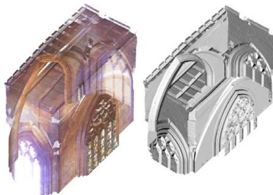
Fig. 3 Point cloud model and mesh model of the north transept
