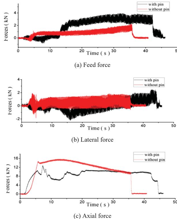
Fig. 5 The effect of pin for forces
