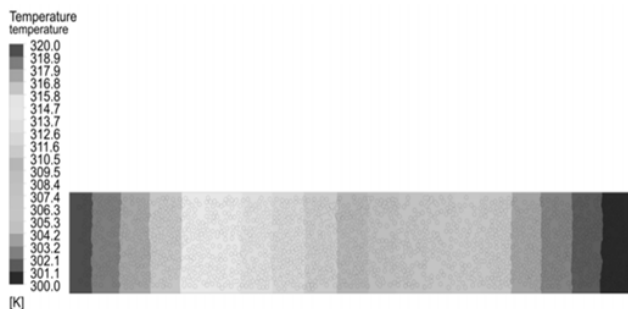
Fig. 9 Numerical computation of thermal conductivity
