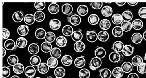
Fig. 5 Detail of the resulting image with highlighted circles representing edges of fibers
