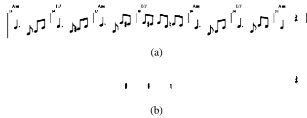
Fig. 10 An example of the accidental and rest recognition: (a) input image; (b) result of the recognition. There is a sharp that is connected with the tail of a musical note, resulting in a recognition failure in our system
