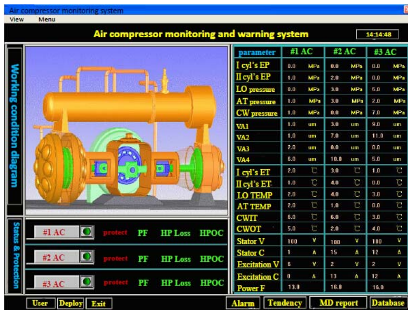
Fig. 8 Main measuring and monitoring interface for air compressor
