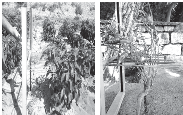
Fig. 2 Manually actuated experimental harvest mechanism
