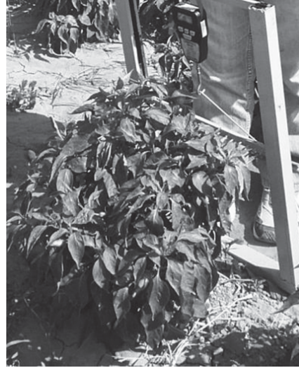
Fig. 3 Force measurements with experimental harvest mechanism
