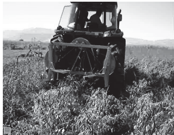
Fig. 11 Harvest experiments with prototype pepper harvest machine
