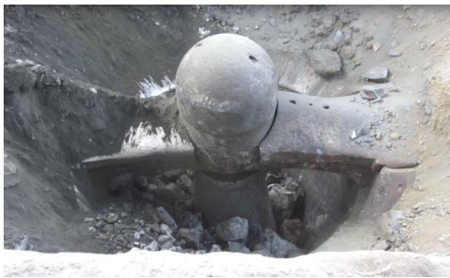
Fig. 6 A view of input of crusher in which charged with iron ore
