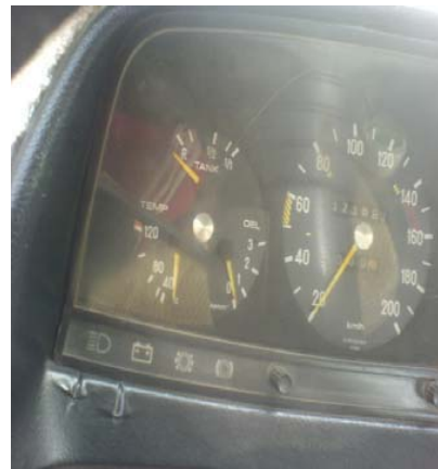
Fig. 2 The analogue fuel gauge of the regular Benz 200 car being investigated
