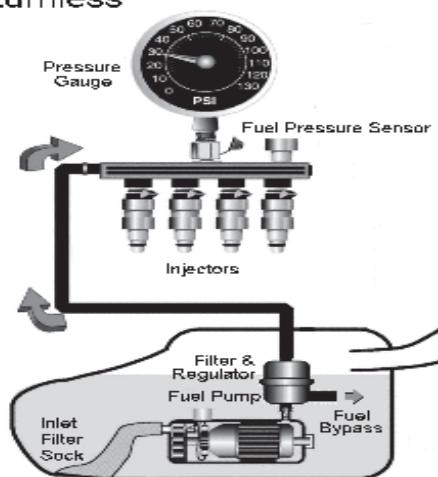
Fig. 1 Return-less flow systems in automobile fuel metering system
