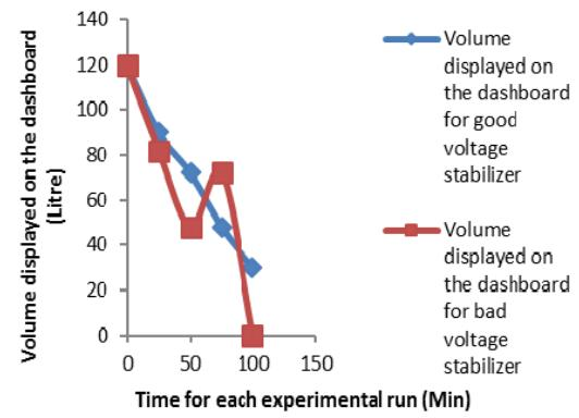
Fig. 4 Plot of volume of ppms displayed on the dash board against time the vehicle has travelled/ worked when voltage stabilizer of the gauge was being investigated
