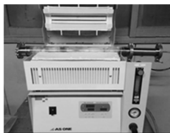
Fig. 1 Lab type electric furnace for sintering process
