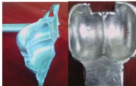
Fig. 9 The defect-free Pelton bucket cast
