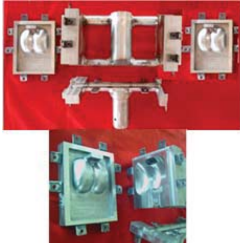
Fig. 3 The fabricated Pelton bucket mould components
