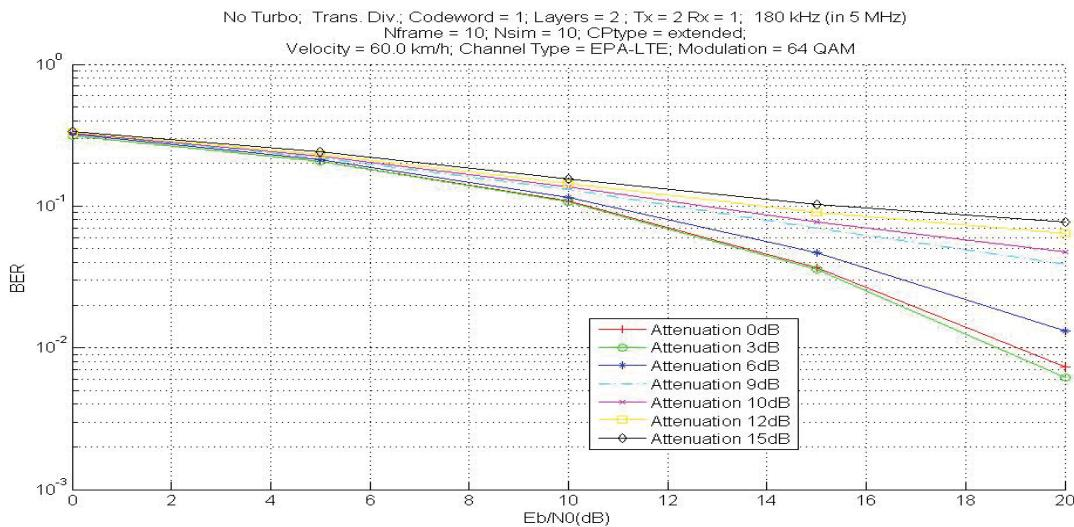
Fig. 4 The simulated effect of hard-clipping CFR on BER at various Eb/No levels for 64-QAM modulation
