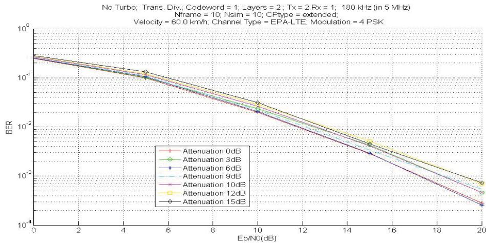
Fig. 2 The simulated effect of hard-clipping CFR on BER at various Eb/No levels for QPSK modulation
