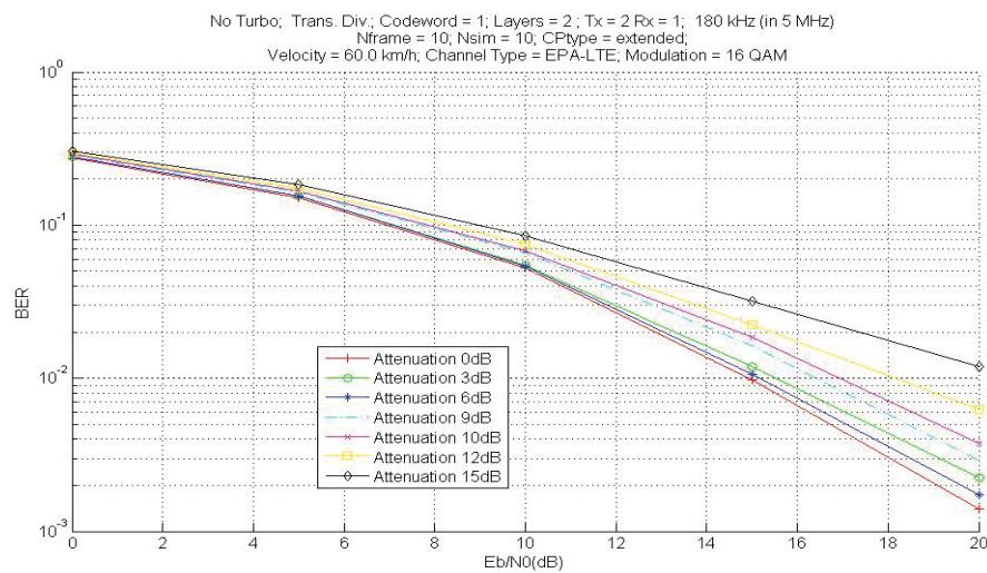
Fig. 3 The simulated effect of hard-clipping CFR on BER at various Eb/No levels for 16-QAM modulation
